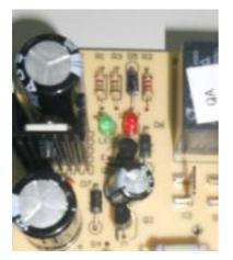
5.3.2 The flash on the outdoor electrical board blinks four times every 5 seconds; it means the phase sequence is wrong
