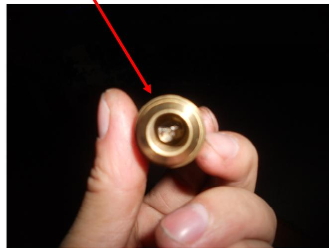
If the high pressure is higher than 2.6Mpa and low pressure is lower than 0.6Mpa, it may be caused by exceeded refrigerant. Then click valve spool of needle valve to release part of refrigerant.
