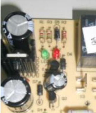
5.3.2 The flash on the outdoor electrical board blinks four times every 5 seconds; it means the phase sequence is wrong
